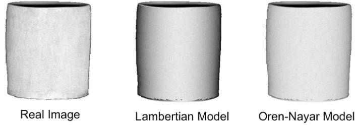
Figure 2: Comparisons between a real image, Lambertian and Oren-Nayar surfaces. [4]
